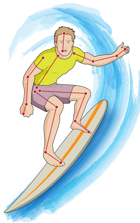
Determining the centre of gravity by segmentation
