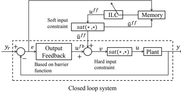
Fig. 1: Block diagram of the proposed control structure
