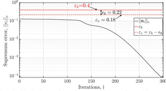
Fig. 5: Variation of supremum norm of tracking error
