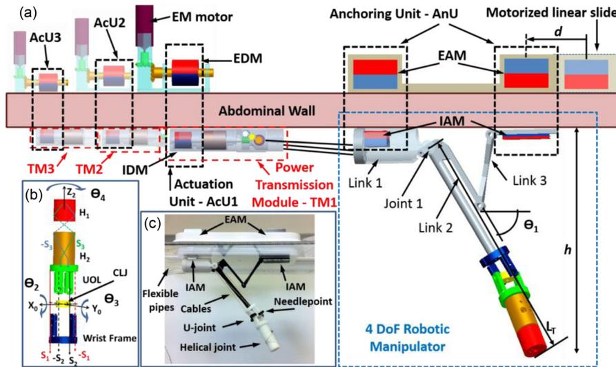
**Fig. 1 (a) Schematic view of the multiDOF-LMA design, (b) the spherical wrist schematic design, and (c) the prototype implementation picture**
