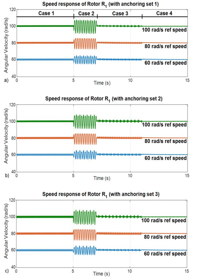
Fig. 5: Simulation results on the LMA system with four cases, including the implementation of  $IMP_{d1}$  (i.e. Case 3) and  $IMP_{d1,d2}$  (i.e. Case 4) for comparisons with reference speeds of 60rad/s, 80rad/s and 100 rad/s on rotor  $R_1$ : a) with anchoring set 1 b) with anchoring set 2, and c) with anchoring set 3.
