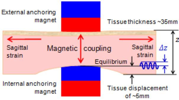
Fig. 3: Schematic diagram of the tissue cross section, illustrating the equilibrium state of the tissue when magnetically “clamped” or anchored. The tissue experiences perturbations in the direction normal to the anchoring axis,  $\Delta z$  about the equilibrium state due to external excitation signals [13]. (Note: the amount of tissue compression in the illustration is exaggerated for visualisation purpose.)
