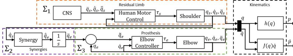
Fig. 2. Synergistic human-prosthesis arm block diagram.
