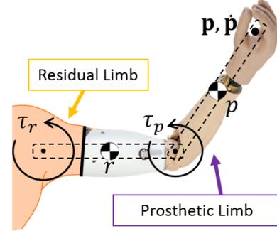
Fig. 1. Human-prosthetic arm diagram.
