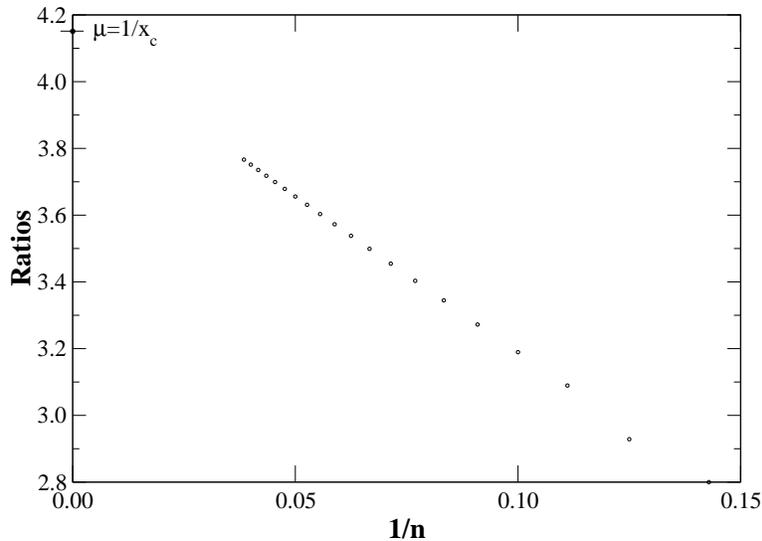
**Fig. 1** Plot of ratios against  $1/n$  for triangular lattice polygons. A straight line through the last few data points intercepts the Ratios axis at  $1/x_c$ .
