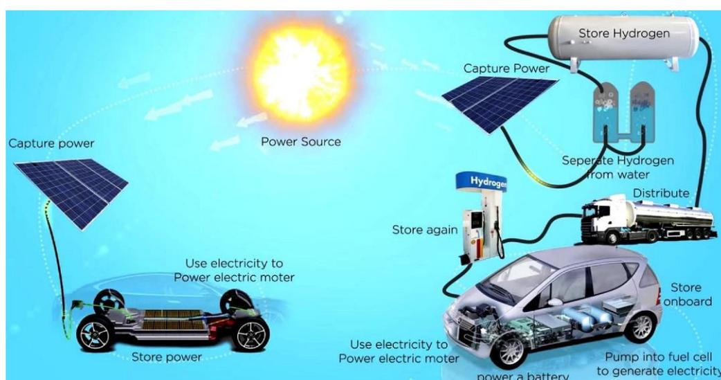
**Figure 1:** Left, power mechanism of battery electric vehicle. Right, power mechanism of hydrogen fuel-cell electric vehicle (Image: [www.aveq.ca](http://www.aveq.ca)).
