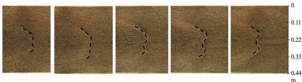
Figure 2. Temporal evolution of an emerging bedform from top view. Flow is left to right and mean flow velocity is 0.43 m/s, the water depth is 0.18 m and the bed slope is 0.0010 m.
