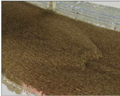
Figure 4. Reconstructed topographic model of the sand bed with the emerging bedform after t_5 , using through-water SfM. The height of the emerging bedform is 0.015 m. Side walls of the flume are presented for scaling.
