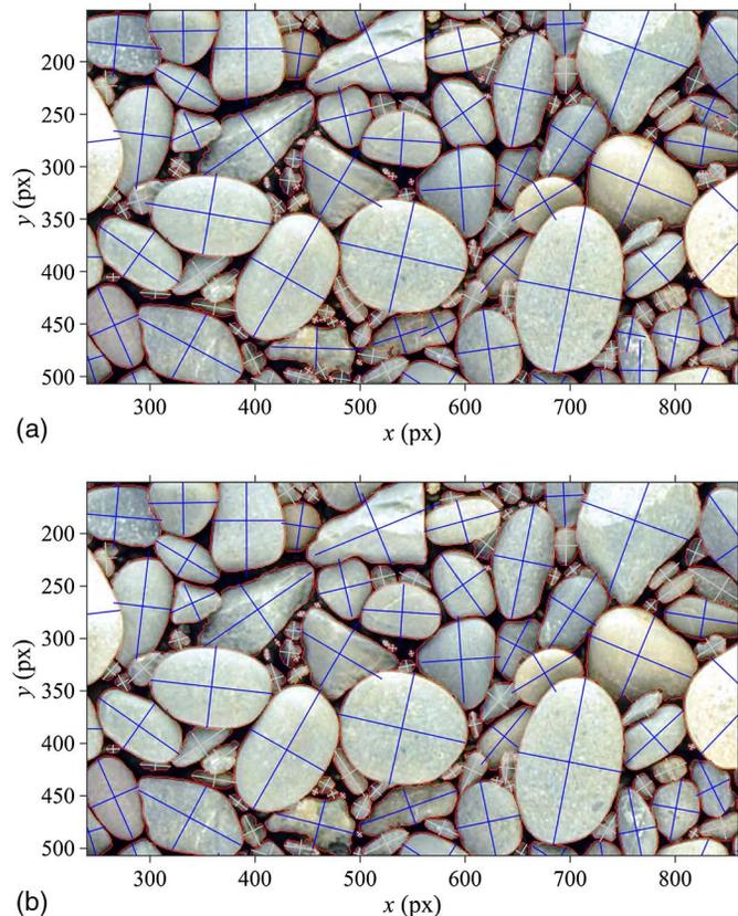
**Fig. 3.** Typical snapshot result of *BASEGRAIN*: (a) before; and (b) after using the manual postprocessing tools; image shows a part of water-worked laboratory flume bed of  $356 \times 620 \text{ px}^2 = 60 \times 105 \text{ mm}^2$ ; only grains with  $a'$ -axes and  $b'$ -axes highlighted in blue (here  $b' > 5 \text{ mm} = 29.6 \text{ px}$ ) are considered in the analysis, while white axes indicate that sizes fall below truncation criterion (here,  $b' \leq 5 \text{ mm}$ )
