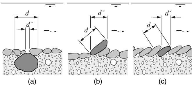
**Fig. 2.** Three potential causes for underestimating real grain sizes  $d$  as apparent grain size  $d'$  as object-detected on top-view photographs (redrawn from Graham et al. 2010, with permission from Wiley, copyright © 2000-2016 by John Wiley & Sons, Inc. or related companies, all rights reserved); grain size  $d$  is represented by intermediate  $b$  axis: (a) burial; (b) foreshortening; (c) overlapping (imbrication)
