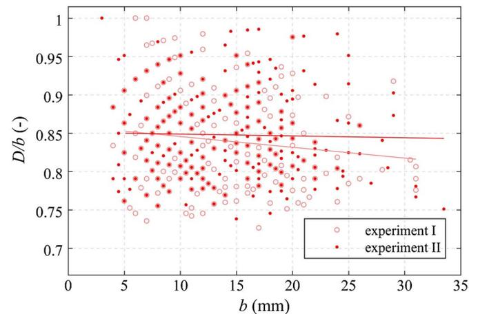
**Fig. 4.** Sieve correction factor  $D/b$  [Eq. (1)] for line-samplings of laboratory Experiments I and II; linear fits to data sets indicate a slight decrease of  $D/b$  towards larger grain sizes
