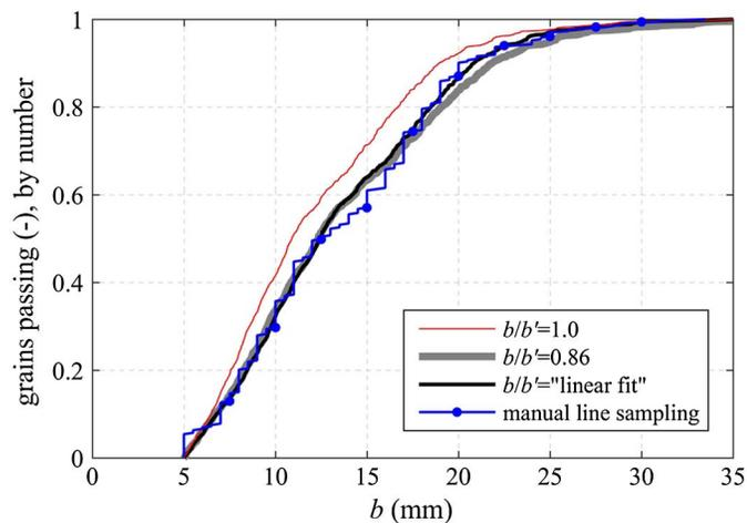
**Fig. 6.** GSDs ( $b$ -axis of grains passing by number along transects) of stones collected in Experiment I (345 grains) and *BASEGRAIN* analysis (1,578 grains for  $b/b' = 1.0$ , and 1,757 grains for  $b/b' = 0.86$ , and 1,799 grains for linear fit, respectively; a higher number of the two latter is due to truncation at  $b < 5$  mm, but  $b \neq b'$ )
