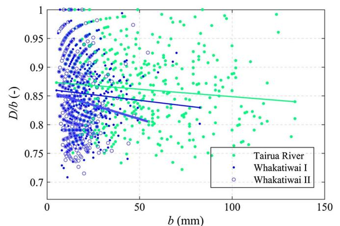
**Fig. 7.** Sieve correction factor  $D/b$  [Eq. (1)] obtained at three field sites; lines show linear fits to data sets; apparent pattern for smaller  $b$  values is due to its discretization to a multiple of 0.5 mm
