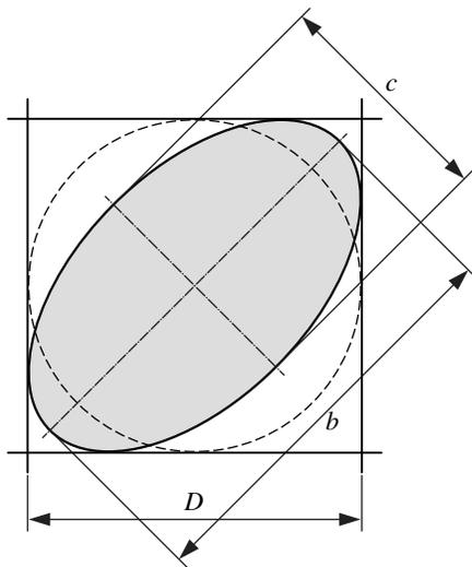
**Fig. 1.** Definition sketch for lengths  $D$ ,  $b$ , and  $c$ , allowing for comparison between grain sizes determined by square-hole sieving and measured with caliper
