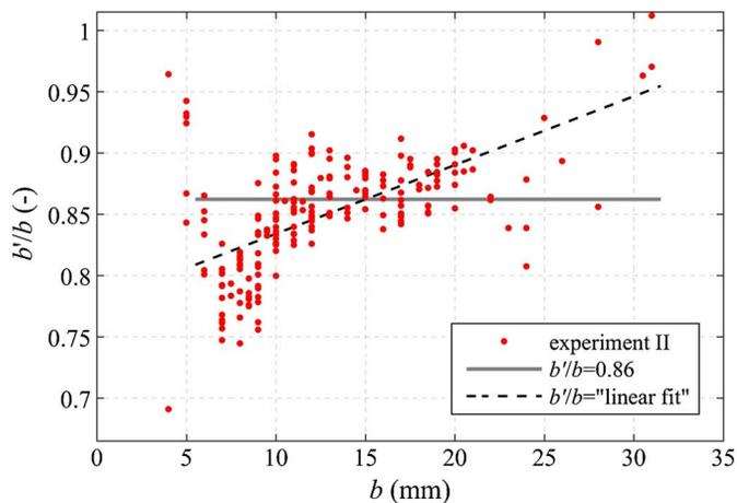
**Fig. 5.** Underestimation of real grain sizes  $b$  inventoried by line-sampling against grain sizes  $b'$  measured by *BASEGRAIN*, both determined during Experiment II
