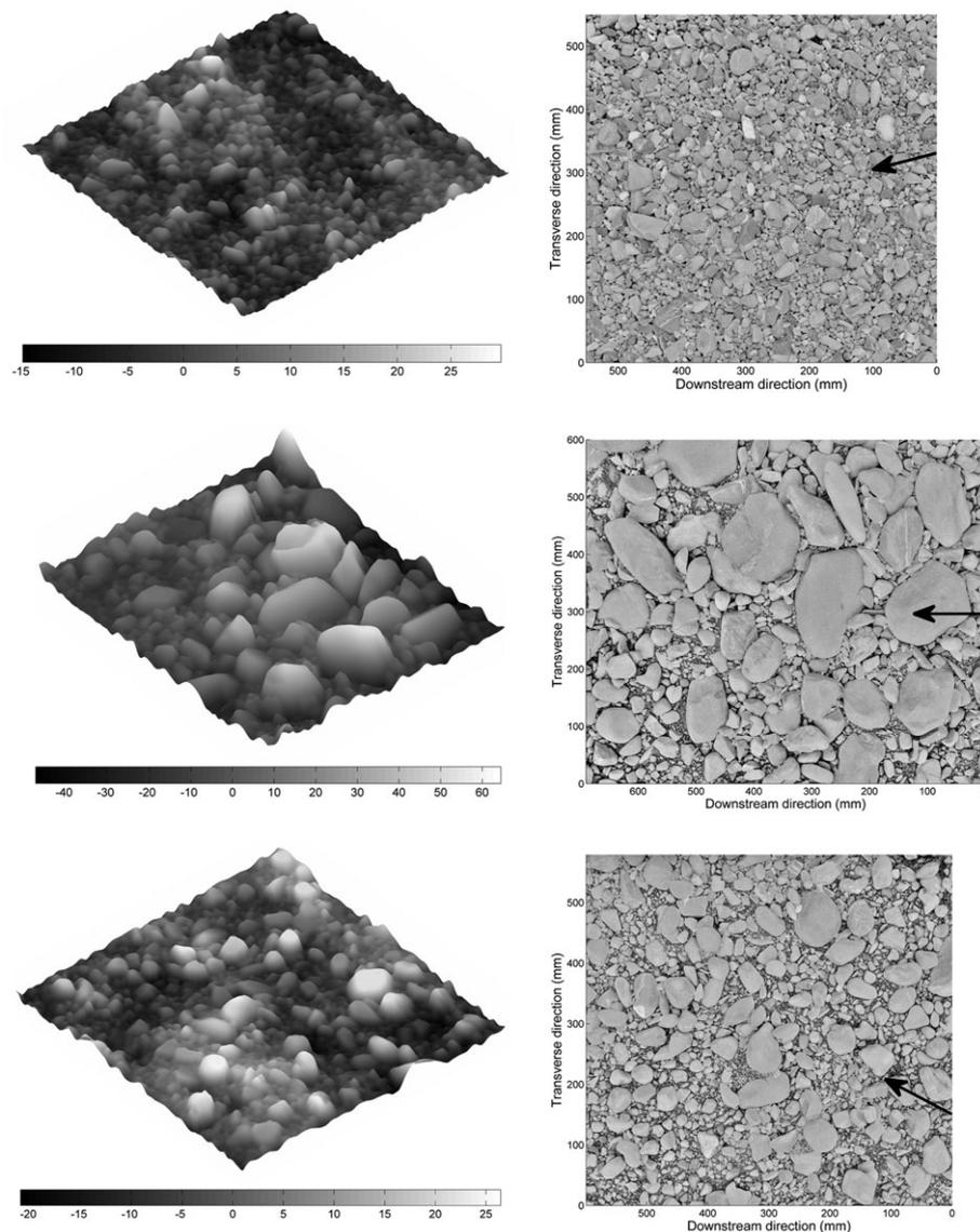
**Figure 3.** Final DEMs and ortho-images from the Whakatiwai patches (bar #1 to bar #3 from top to bottom). Elevation is represented as gradient of greys, and is in millimetres. Flow direction, determined visually in the field, is from right to left. Arrows show the most probable flow direction (Figure 8).
