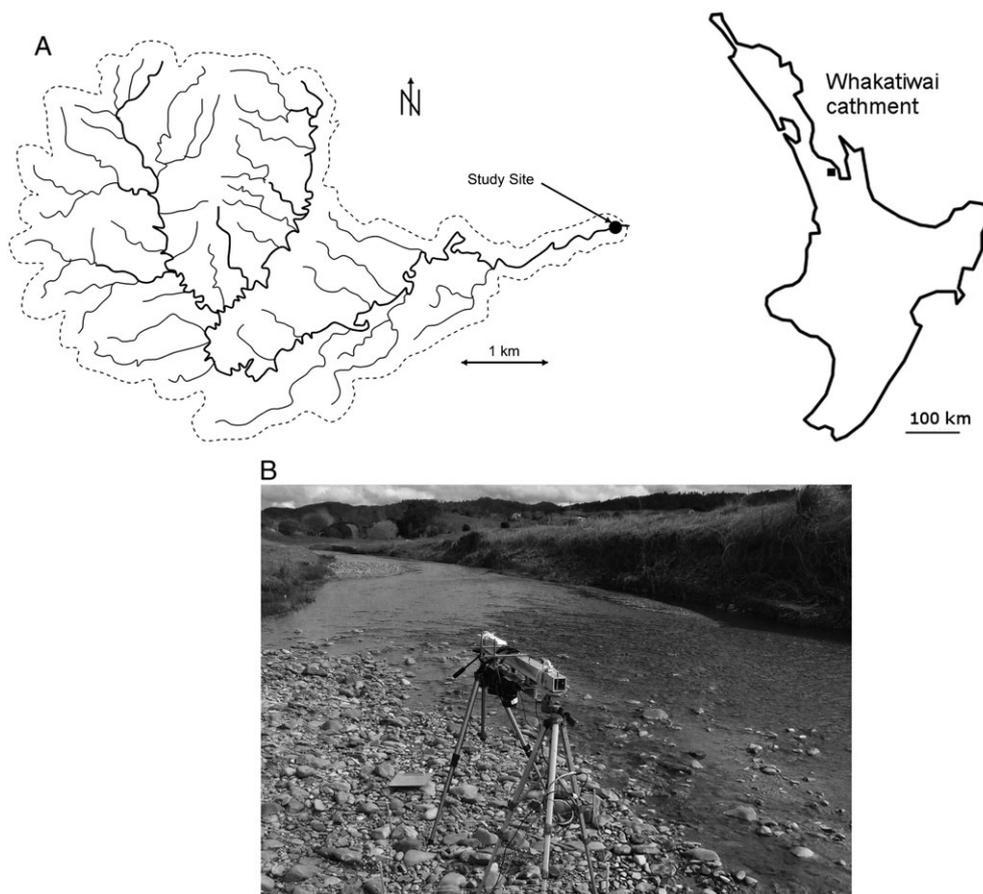
**Figure 1.** Whakatiwai catchment in the North Island of New Zealand. (A) Site location. (B) Image of CRDP deployment on bar #2, looking upstream. Note the alignment of the setup with the apparent flow direction.
