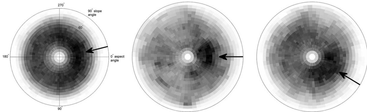
**Figure 7.** Polar plots of all 1 mm<sup>2</sup> DEM grid cells aspect and slope angles for the three patches (bar #1 to bar #3 from left to right). Aspect angle is from 0° to 360° and slope angle is from 0° to 90°; plots are shaded by point density (high density in black, zero density in white). The assumed flow direction is from 0° to 180°. Arrows show the most probable flow direction, based on Figure 8.
