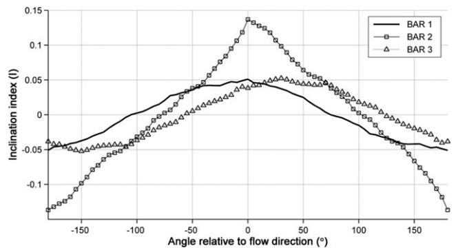
**Figure 8.** Directional inclination indices for the three patches. Inclination was calculated for all angles between –180° and 180° at a 5° interval, using a separation distance between pairs of points of 1 mm, which is the DEM sampling distance, the lag for which imbrication was the most perceptible.
