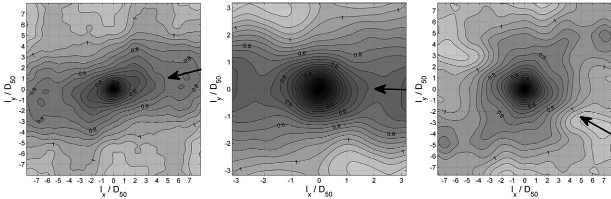
**Figure 6.** Two-dimensional isopleth maps of the generalized second-order structure functions for the three patches (bar #1 to bar #3 from left to right). The assumed flow direction is along the horizontal axis. Arrows show the most probable flow direction, based on Figure 8.
