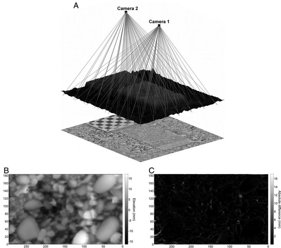
**Figure 4.** (A) Close-up presentation of on-site quantitative evaluation of CRDP performance using a 3D-printed gravel-bed model. (B) Measured DEM of the 3D-printed model. (C) DEM of difference (DoD) between measured and truth data (0.25 mm sampling distance).
