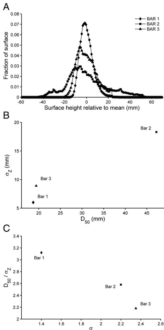
**Figure 5.** (A) Distributions of surface elevations for the three patches. (B) Relationship between the standard deviation of bed elevations ( $\sigma_z$ ) and the bed-surface  $D_{50}$ . (C) Relationship between  $D_{50}/\sigma_z$  and the sediment geometric sorting ( $\sigma$ ).
