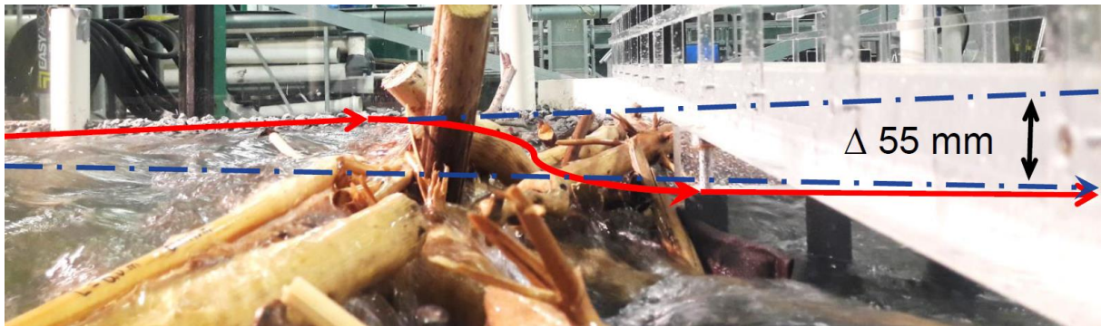
Figure 3. Side view - observed backwater effect (in red the backwater influenced water level, in blue the normal water level).
