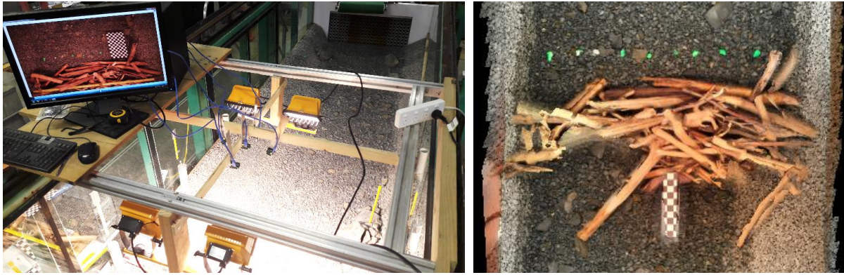
Figure 2. SfM setup (left,a) and orthophoto of LWD accumulation captured with SfM (right,b).
