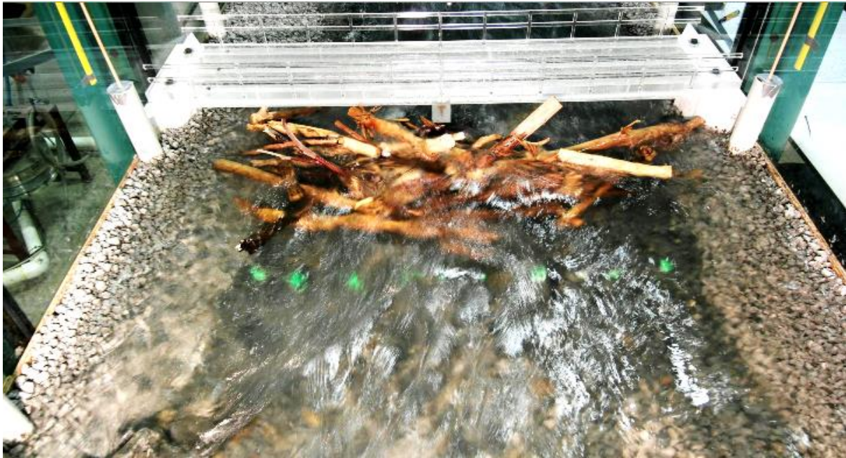
Figure 1. Plan view of LWD accumulation in our laboratory setup.
