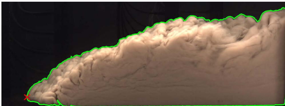
Figure 1. Vector delineation of an image from experiment N2 using the thresholding technique. The identified frontal boundary of the current is shown by the red 'x'.
