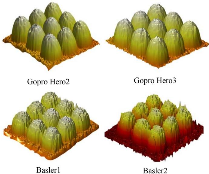
Fig. 8. The reconstructed DEMs based on the ‘centre’ calibration case for ‘C’ camera to object distance.
