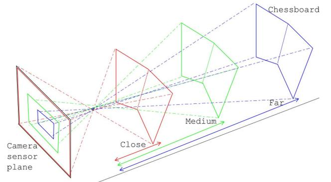
Fig. 3. Effect of changes in target to camera distance for Tsai’s calibration.
