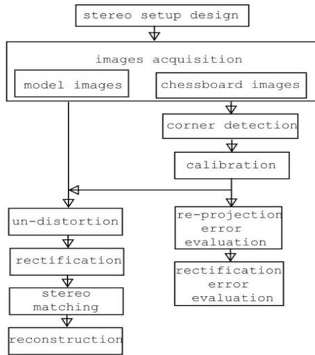
Fig. 1. General stereo-vision pipeline.
