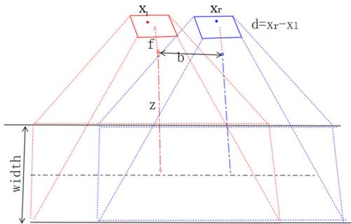
Fig. 2. Stereo-vision setup.
