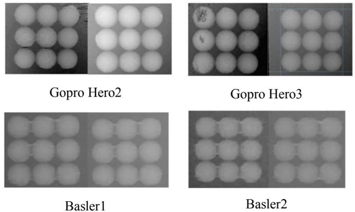
Fig. 7. Depth map results for ‘whole’ and ‘centre’ calibration targeted case for each tested camera configuration ‘Whole’ is the left image of the pair, and ‘centre’ is the right image of the pair.
