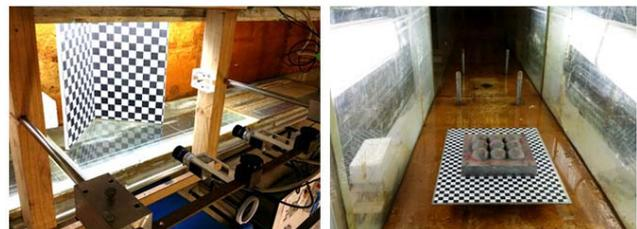
Fig. 4. Experimental setup in the hydraulic flume with Tsai calibration target (left) and lighting setup with two 1 m long neon lights placed at both sides of the flume (right).
