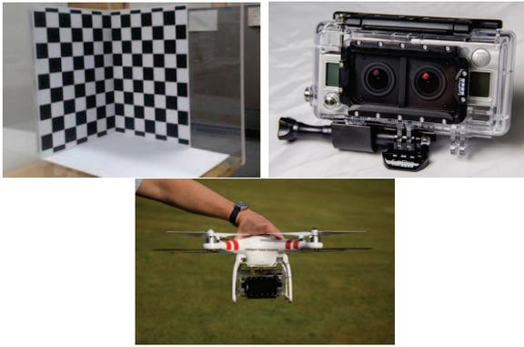
Figure 1. Zhang calibration Object (Top Left), GoPro HERO3+ Cameras (Top Right), Phantom quadcopter (Bottom Middle)
