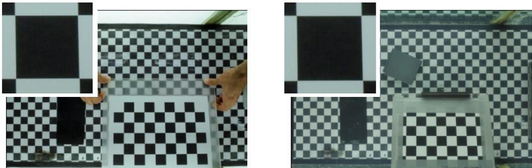
**Figure 2** Left-camera image of the checkerboard obtained in air with setup 1 (left) and with 200-mm water depth with setup 5 (right) with a zoom on the red-squared corner. In the background is the large checkerboard used for mechanical alignment, which also protected the gravel-bed during the calibration.
