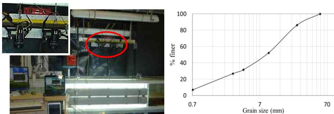
**Figure 1** The photogrammetric setup (left) and particle size distribution from size sieving (right).
