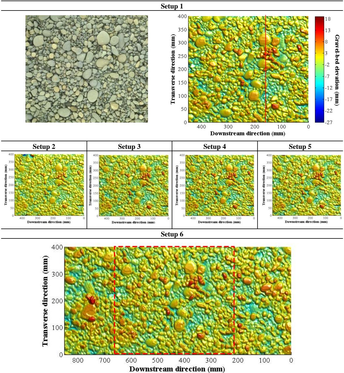
**Figure 4** Photograph of the small measurement window and detrended DEMs obtained with setups 1 to 6. The same color mapping was applied to all DEMs to facilitate the visual comparison. The red line in the DEM of setup 1 shows the location of the transverse profile as seen in Figure 3.
