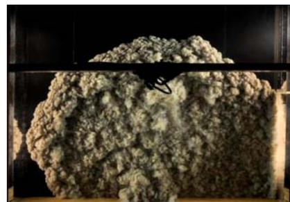
Figure 4. Typical 2-D propagation of an unconfined turbidity current. Note the upward transport and reflections at the left hand side wall.
