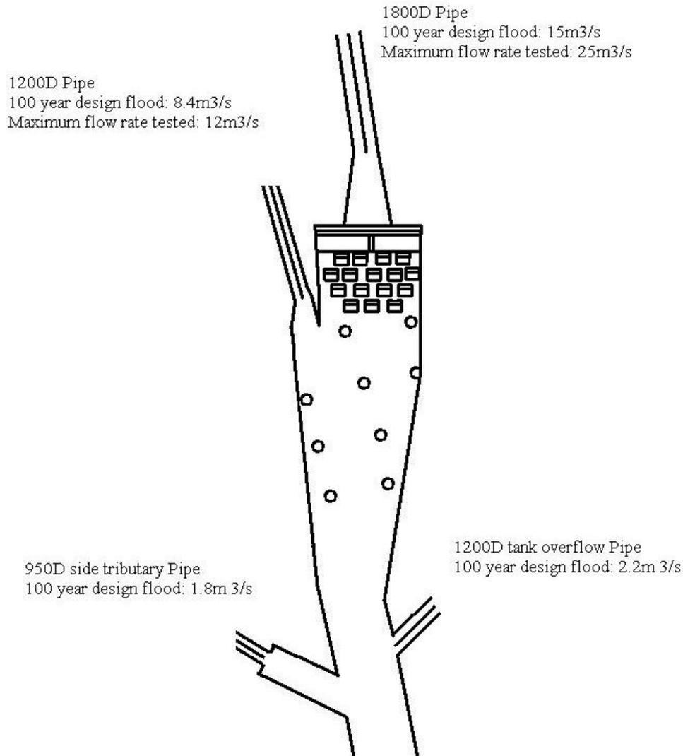
**Figure 3: Schematic overview of outlets and flow rates**
