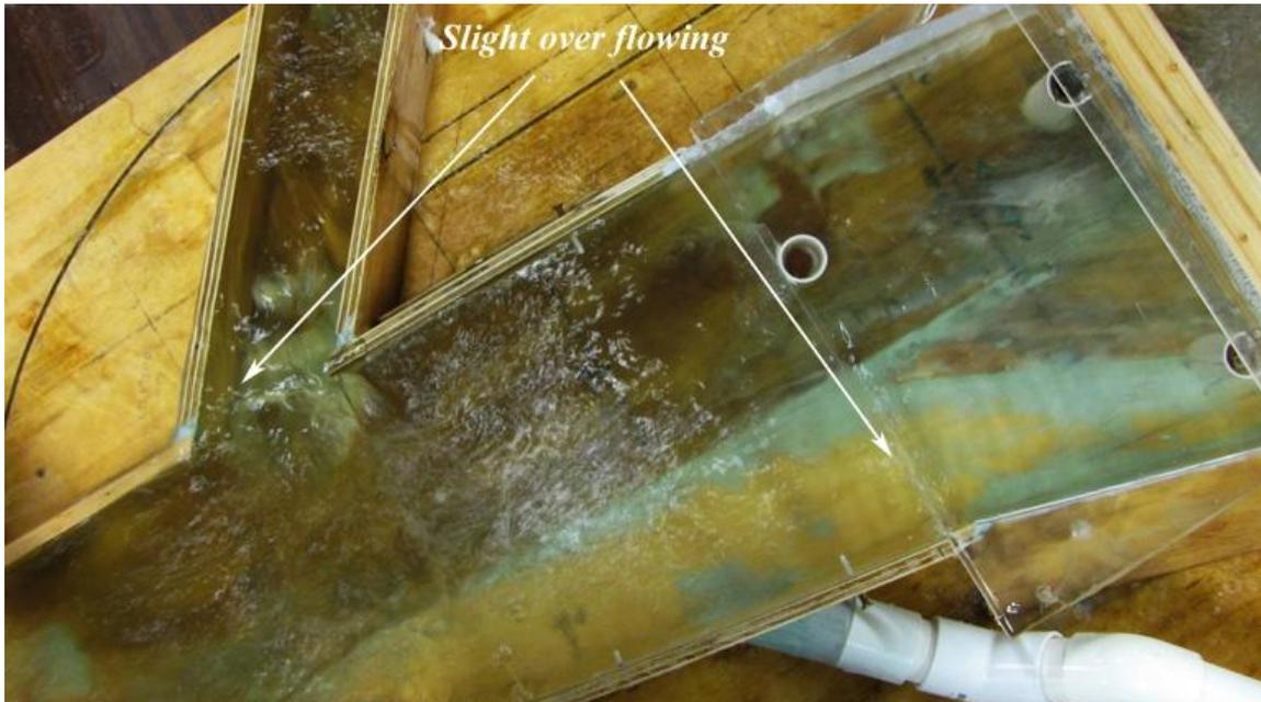
**Figure 5: Overflowing at maximum flow rate ( $41\text{m}^3/\text{s}$ )**
