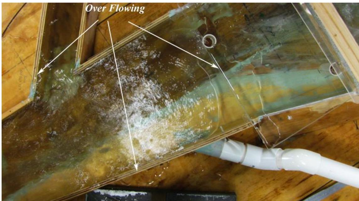
**Figure 6: Overflowing at maximum flow rate ( $41\text{m}^3/\text{s}$ ) with weir**
