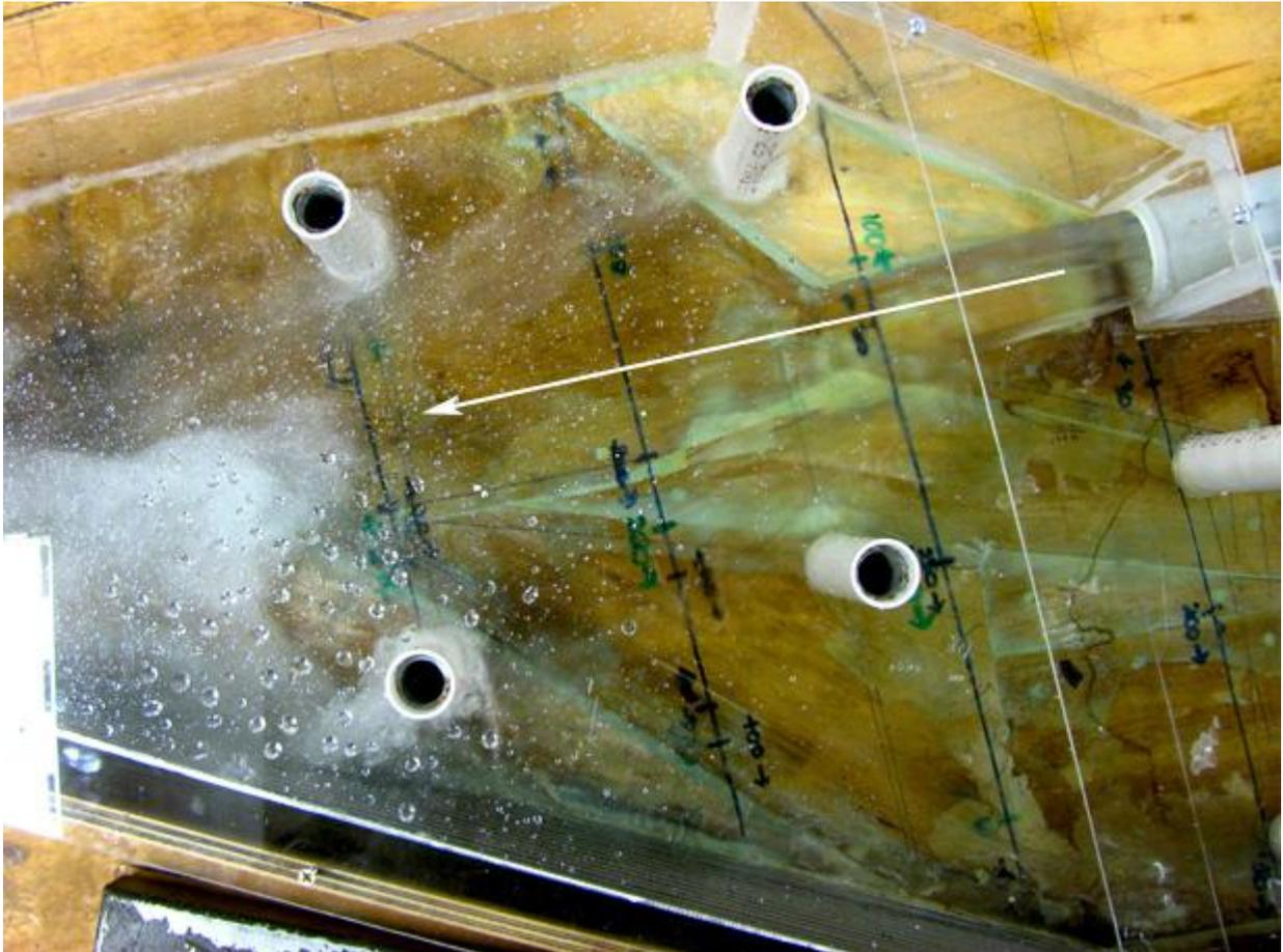
**Figure 4: Jet of water forms in the 1200Ø pipe. Best seen at flow rate of 8.4m<sup>3</sup>/s (0m<sup>3</sup>/s in the 1800Ø pipe 8.4 m<sup>3</sup>/s in the 1200Ø pipe)**
