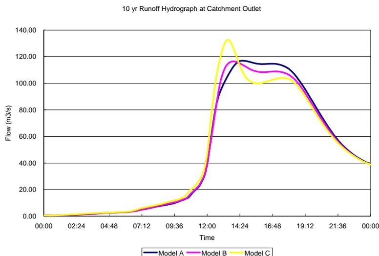
**Fig 5. 10 yr Runoff Hydrograph at Catchment Outlet Produced by Model A, B and C.**
