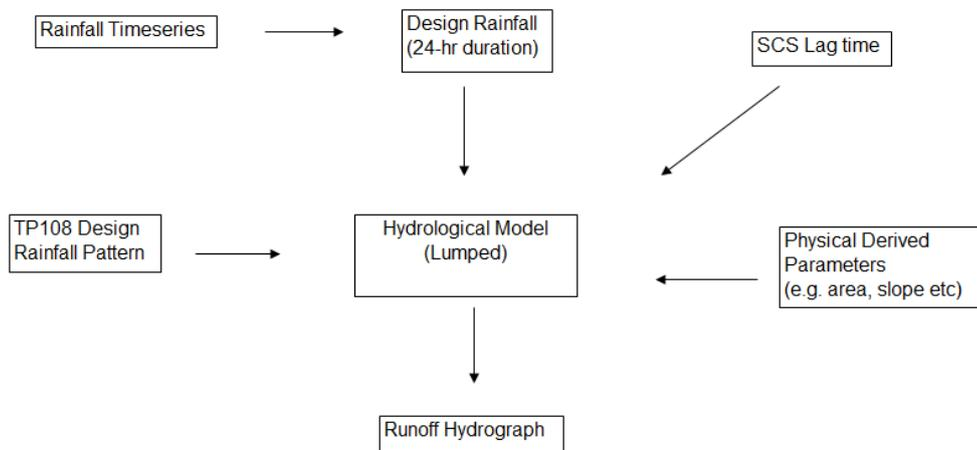
**Fig 2. HEC-HMS Hydrological Modelling Flow Chart**
