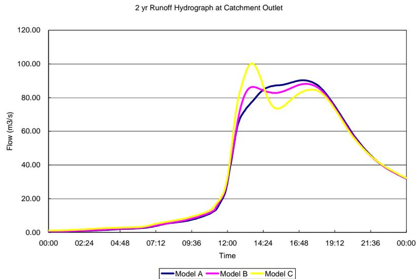
**Fig 4. 2 yr Runoff Hydrograph at Catchment Outlet Produced by Model A, B and C.**
