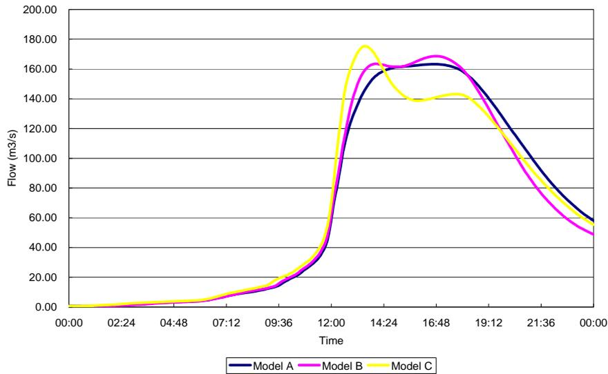
**Fig 6. 100 yr Runoff Hydrograph at Catchment Outlet Produced by Model A, B and C.**
