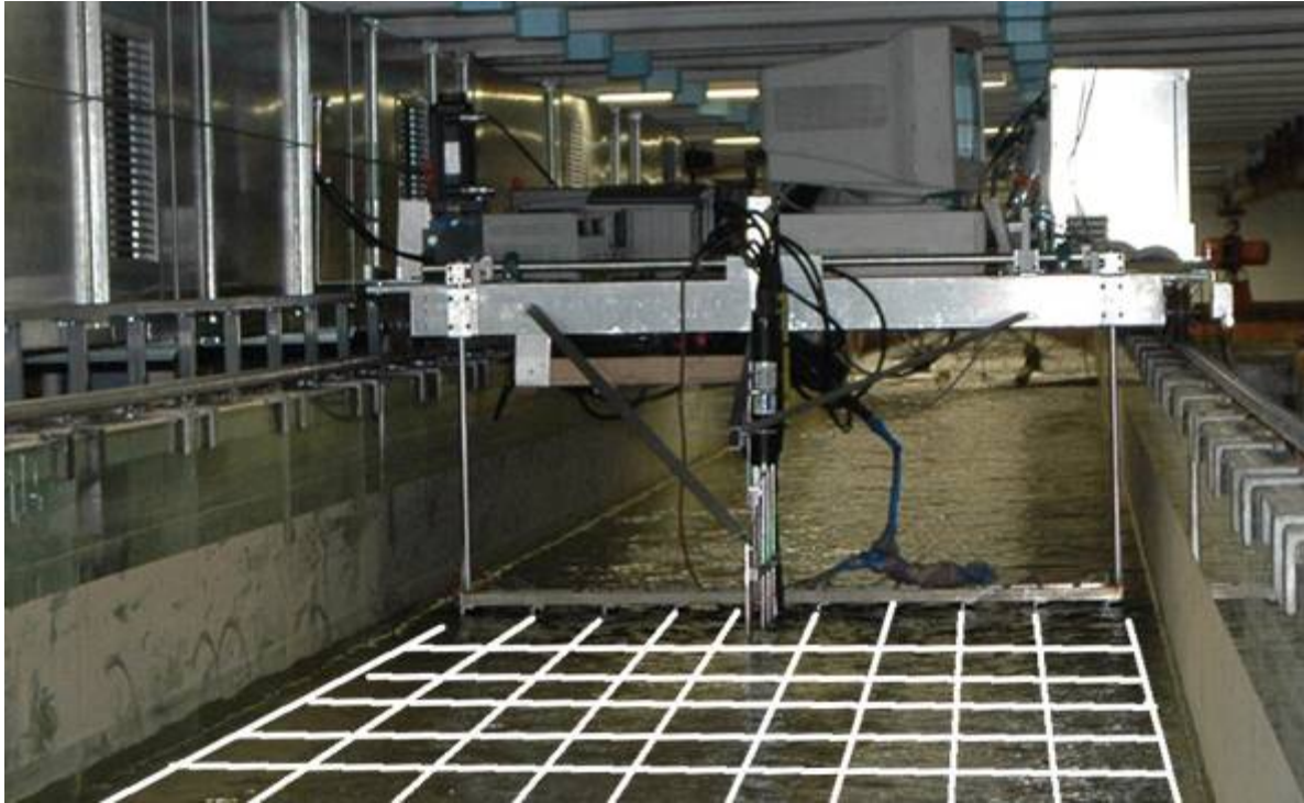
Figure 3 Schematic display of sand-bed elevation recording grid in the 5-ft flume. The carriage travels downstream (for recording) and upstream (with the sensors out of the water) along the flume over a length of 18.48-m.
