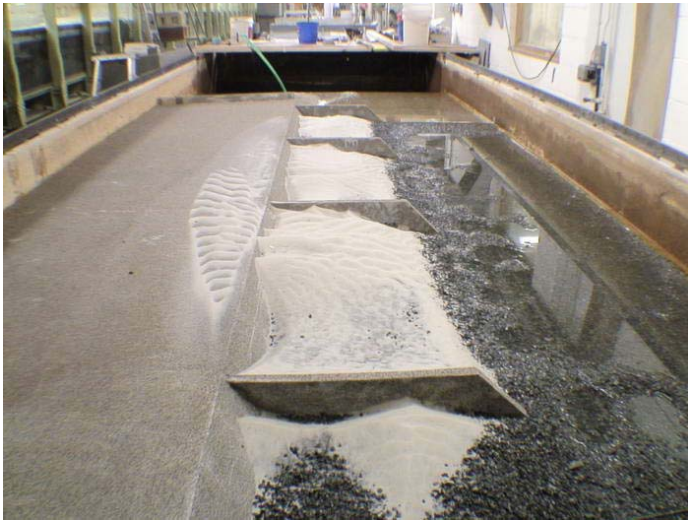
Figure 1. Wide flume used for the study. Downstream view. From left to right: floodplain, four groynes, main channel.
