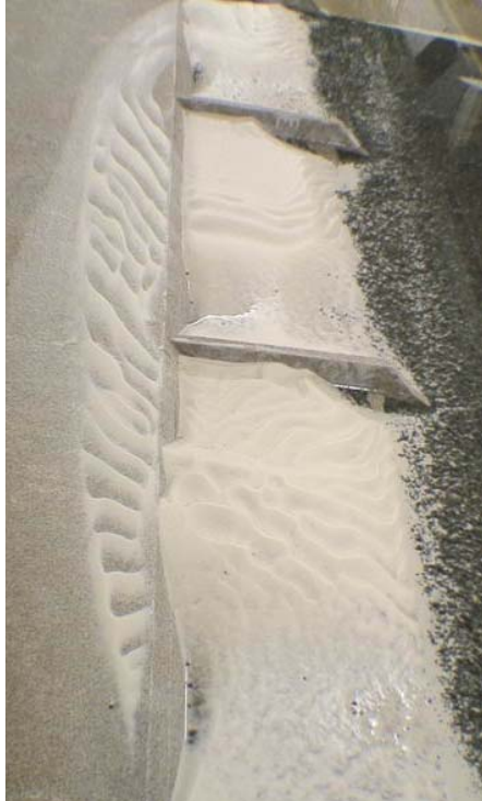
Figure 4. Top view of groynes two to four. Flow is from bottom to top. Main channel on the right and floodplain on the left.
