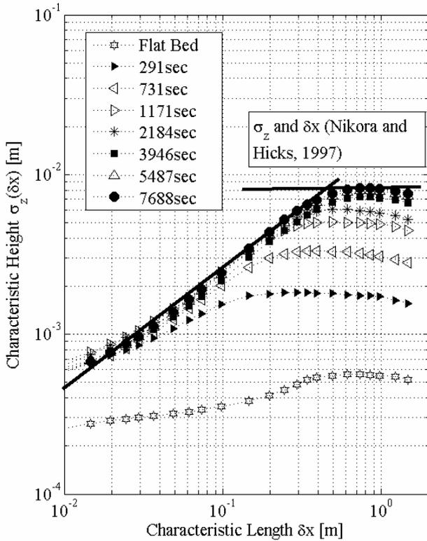
Figure 5. Exemplary functions  $\sigma_z(\delta x, t)$  for experiment T3 during dune development starting from a flat bed. The self-similarity of dunes is characterized by the similar slopes in the scaling region after initial dune development.
