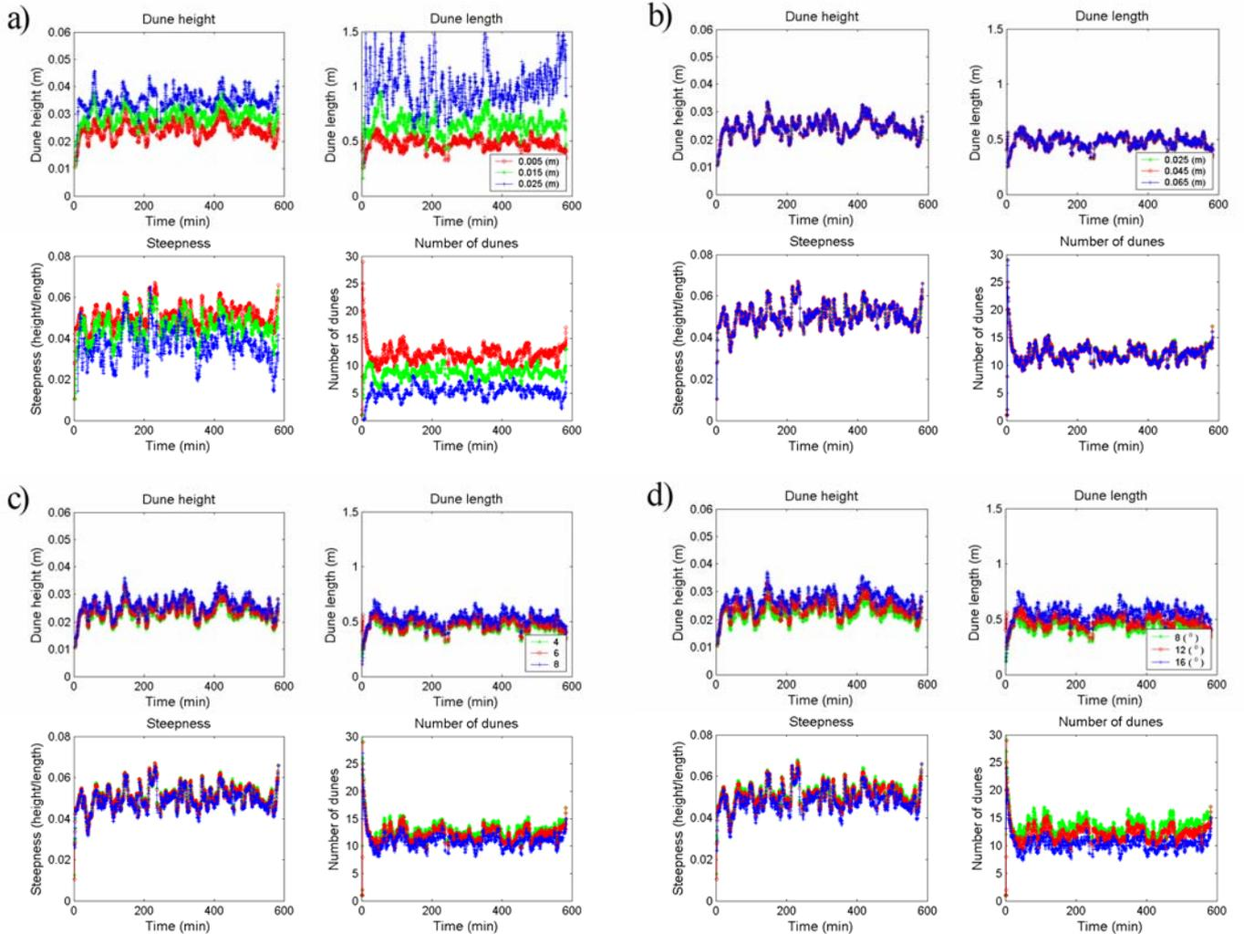
Figure 3. Discrete bed-form statistics of experiment T14. a) Change in threshold for dune height; b) change in threshold for allowable horizontal separation distance between identified lee-face points; c) change in threshold for number of sample points of lee face; d) change in threshold for angle of lee face.
