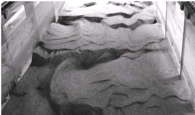
Figure 2. Irregular 3D dunes as generated in a wide 1.5-m wide flume. Flow is from top to bottom. Superposed sand sheets are clearly visible.  $D_{50}=0.85$ -mm.
