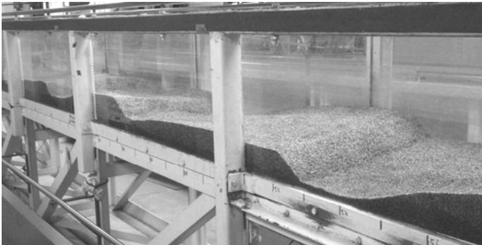
Figure 1. Roughly 2D dunes as generated in a narrow 0.44-m wide flume. Flow is from left to right.  $D_{50}=0.85$ -mm.
