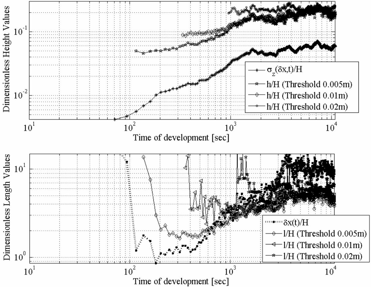
Figure 6. Relationship of averaged dimensionless discrete height  $h/H$  and length  $l/H$  values (different minimum dune height thresholds are applied) and dimensionless characteristic height  $\sigma_z(\delta x, t)/H$  and length  $\delta x(t)/H$  values during dune development.  $m$  (Eq. 1) does change significantly during dune development (see also Figure 7). The development is shown for the first 3-hrs for experiment T3.
