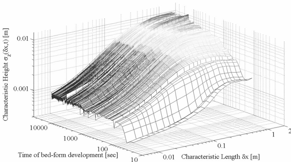
Figure 4. Development of characteristic height  $\sigma_z$  and characteristic length  $\delta x$  during dune development (here shown for experiment T13). It shows the initial fast development of the characteristic height  $\sigma_z$ , as well as the asymptotic approach of the characteristic length  $\delta x$  towards a saturated value during development of an equilibrium dune bed.
