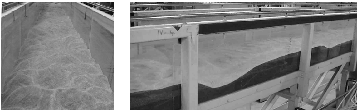
Figure 1 Ripple (left) and dune (right) beds in as seen in the 0.44-m wide flume at the University of Auckland.
