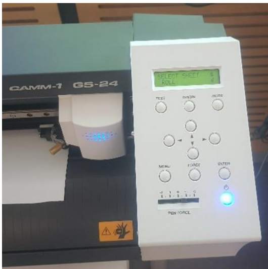
Figure 4: Roland GS-24 Vinyl Cutter Turned On and Calibrated
