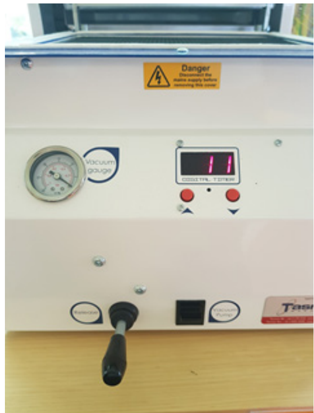
Figure 8: The 3 switches clearly labelled on the machine, as well as the adjustable timer
