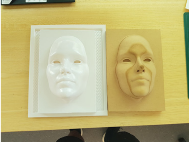
Figure 9: A successful vacuum form
