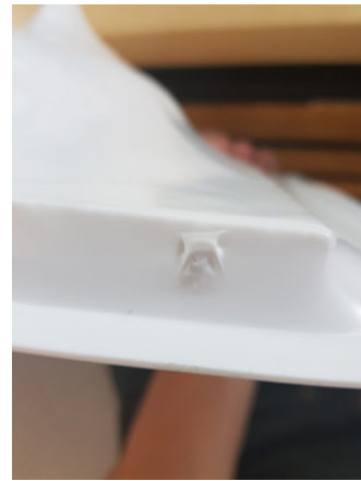
Figure 12: The small tear that caused figure 10 to fail
