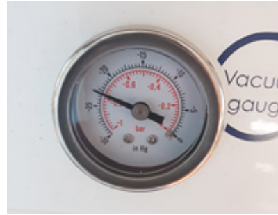
Figure 7: A properly pressurised vacuum chamber, able to suck the plastic to form
