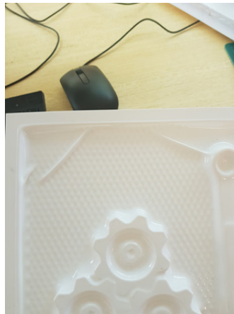
Figure 13: Folds caused by excess heat
