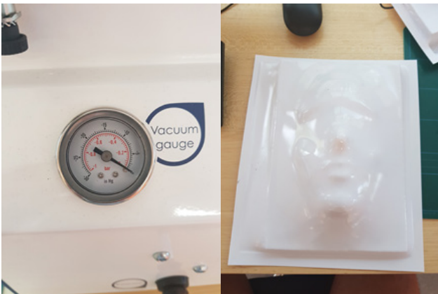
Figure 10,11: a failed vacuum form, due to lack of suction
