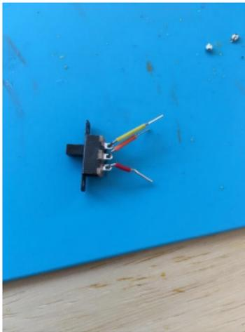
Figure 5: Jumper wires placed in the Switch terminals
