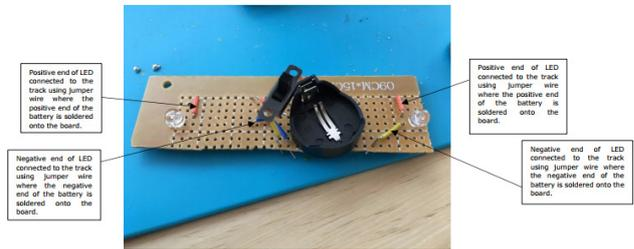
Figure 8: The two orange wires at the extreme ends of the board connect the positive ends of the LEDs to the Positive terminal of the battery while the blue wire on the left side and the yellow wire on the right side connect the negative terminals of the LEDs to the negative terminal of the battery.
