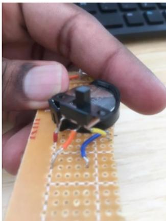
Figure 7: Switch terminals soldered onto the Vero board.
