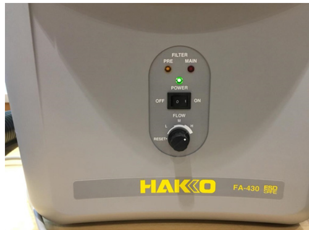
Figure 3: Extraction Unit switched on with maximum extraction settings.
