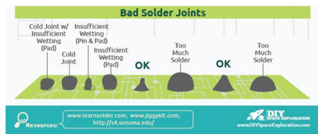
Figure 10: Bad and good solder joints
