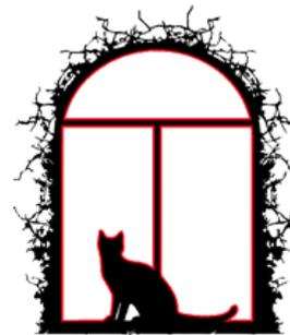
Figure 4: RGB Red lines will be cut & Black lines will be engraved
