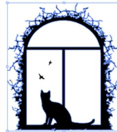
Figure 3: RGB Blue lines will be etched & Black lines will be engraved
