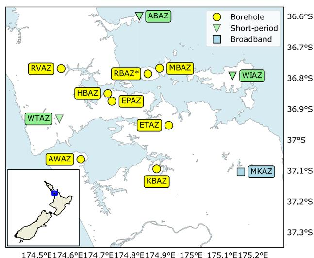
**Figure 1.** The Auckland volcanic seismic network (AVSN) with an additional seismometer from the University of Auckland (RBAZ\*). (Inset) Location within New Zealand. The color version of this figure is available only in the electronic edition.
