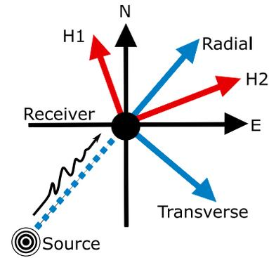
**Figure 2.** After Zha *et al.* (2013), seismometer components and their relation to seismic signals. North (N) and east (E) would be the conventional installation orientations. H1 and H2 represent unknown orientations. For the ambient seismic noise (ASN) orientation method, the source is a different seismic station. For the  $P$ -wave orientation method, the source is an earthquake. The color version of this figure is available only in the electronic edition.
