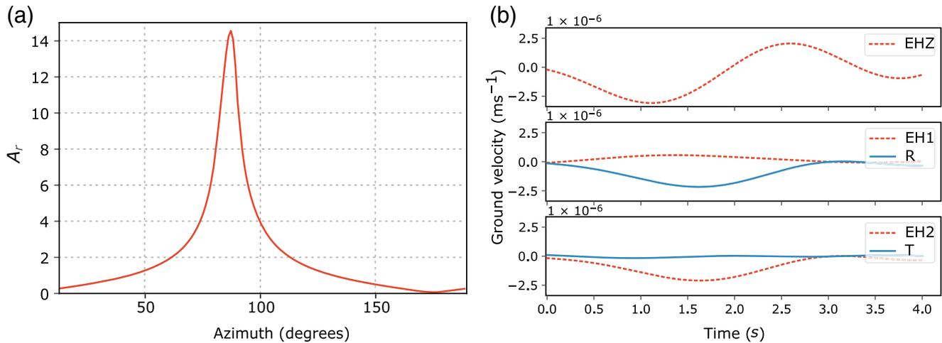
**Figure 4.** (a) The maximum of  $A_r$  corresponds to the orientation of the EH1 sensor in the radial direction. (b) Initial  $P$ -wave signal before and after a rotation maximizing  $A_r$ . (Time is measured from the start of the pick.) The color version of this figure is available only in the electronic edition.
