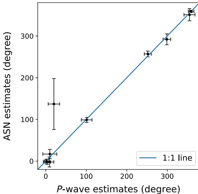
**Figure 7.** ASN-based station orientation estimates and *P*-wave estimates show a correlation coefficient of 0.9699 (excluding the outlier KBAZ, the correlation increases to 0.9994). The color version of this figure is available only in the electronic edition.
